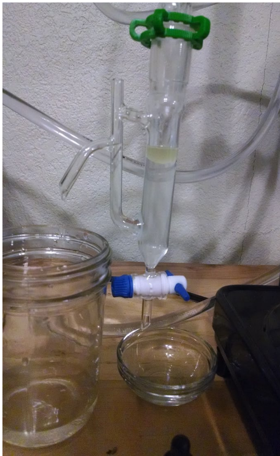
Bottom of condenser, top of water-oil separator: (After about an hour, you can see the essential oil (yellowish) in the water-oil separator):
