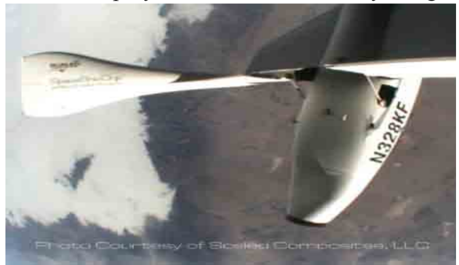
Tail position rotated up 90 degrees for re-entry
