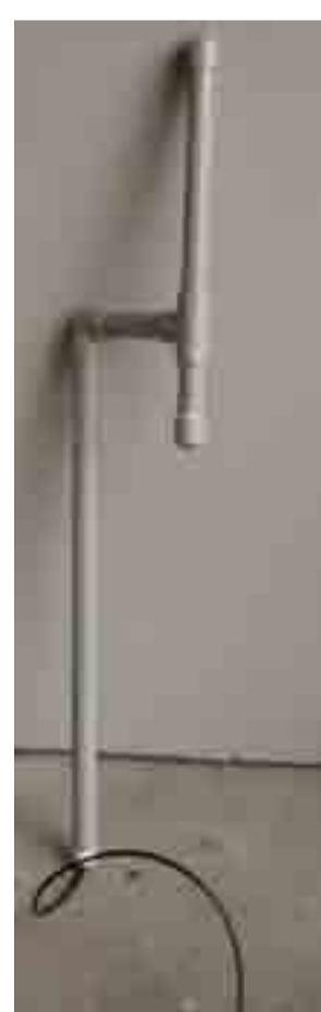
Rubber ducky antenna inside a PVC housing.
