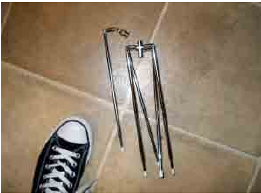
Disassembled 1/4 wave antenna.
